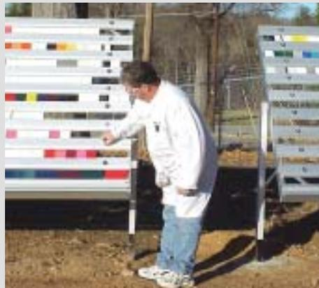
Removing a panel for color testing after weathering.
